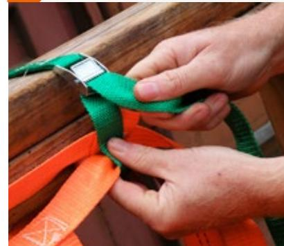
Once you have the net fully erected pull the cam buckles up tight but **not too tight as to deflect frames**.
