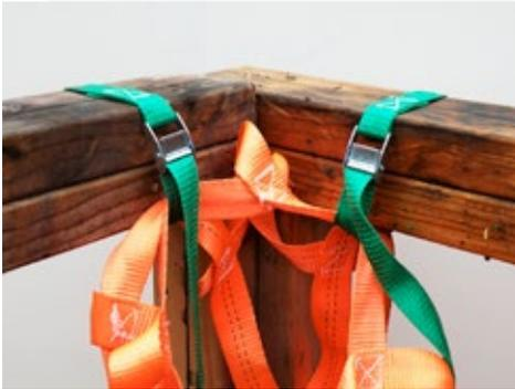
**Attach 1 strap each side of the corner** 150mm from the corner (*for 2 total straps per corner*).
